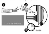
Before inserting the HGT heater into the radiator, a small amount of Loctite Adhesive (included) should be smeared over half of the circumference of the thread. DO NOT put Loctite on the conical gasket, AVOID CONTACT WITH THE SKIN
