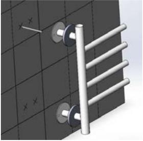
Unthread the cap to see the visible mounting seat, level the installation mounting size and mark installation holes by pencil
