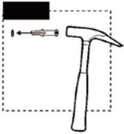
Use a hammer to knock plastic wall anchor into wall completely
